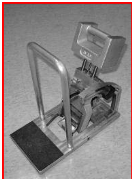
Brungraber Mark II (PIAST) Output = “slip resistance value”
