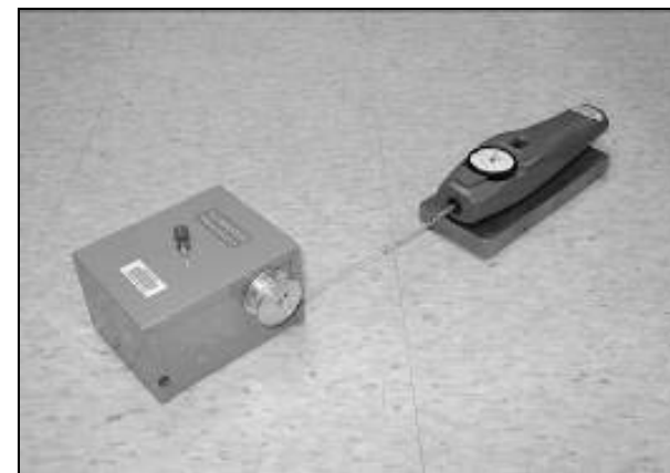
Horizontal Pull Slipmeter (HPS) ASTM F609 Output = “slip index”
