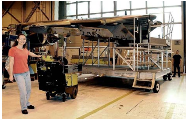
Moving equipment and aircraft parts with the CartCaddy requires only two operators and eliminates ergonomic injuries.
