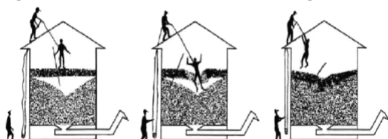
The person on the inside of the bin is secured to the outside of the bin. The person on the roof can pass instructions and assist in lifting. The person on the ground can go for help or assist in pulling.
