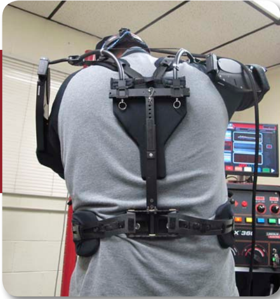
Photos 1 and 2: Vermeer welders during testing with the exoskeleton.
